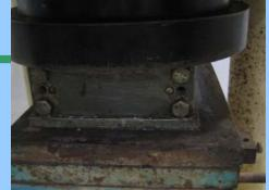
Further compaction using a compression machine at a rate of 600 kN/min twice
