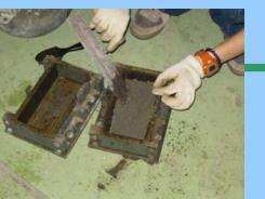
Steel moulds for fabrication of blocks
